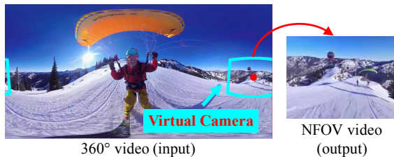
Figure 1: Input and output of the Pano2Vid problem. The task is to control a virtual camera in the 360° camera axis in order to capture a normal video that looks as if captured by human videographer.
