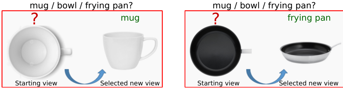
Fig. 2: A schematic illustrating the active categorization of two objects. A moving vision system may not recognize objects after just one view, but may intelligently choose to acquire new views to disambiguate amongst its competing hypotheses.
