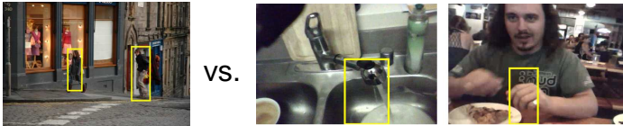
Fig. 2. Understandably, while proficient for human-taken photos (left), today’s best object detectors break down when applied to egocentric video data (right). Each image displays the person detections by the DPM [8] object detector.
