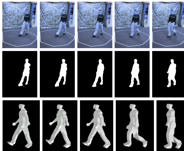
Fig. 7. Example result on real sequential data. Top row shows input sequence, middle row shows extracted silhouettes, and bottom row (output) shows VH hypotheses lying on the ML path, rendered here from a side view of the person in order to display the 3D quality of the estimate.
