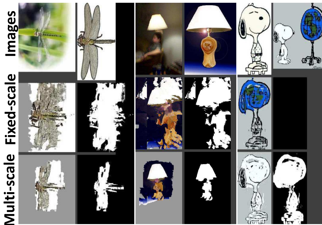
Figure 6.10: Example matching results by my multi-scale matching. For comparison, I also show results from my fixed-scale version. My multi-scale method successfully finds the correct scale between objects, providing accurate matching. On the other hand, a single-scale one prefers the fixed size between objects, causing gross errors: e.g., in the 3rd example, Snoopy matches to a globe since they have similar size.
