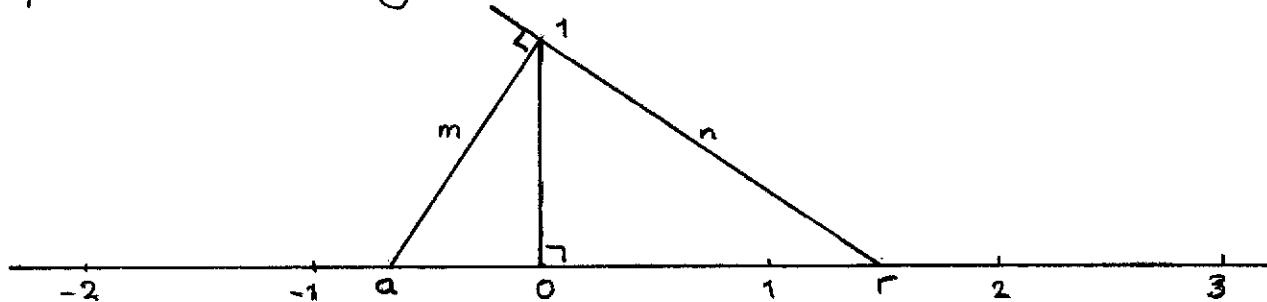
The graphical solver works as follows. From point  $a$  on the horizontal axis, draw the line  $m$  through point 1 on the vertical axis; line  $n$ , through that point and orthogonal to  $m$ , intersects the horizontal axis in point  $r$ .
