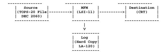
The testing at PAX was done in the following configuration. OSIS was used as the source, and terminals were used for the destination and log. The MFM was not connected to any real destination system. The tests at PAX were the tests developed independently by SDC [Neely 82]. In this configuration, the proved MFM performed correctly in all of the SDC tests on the first attempt.
