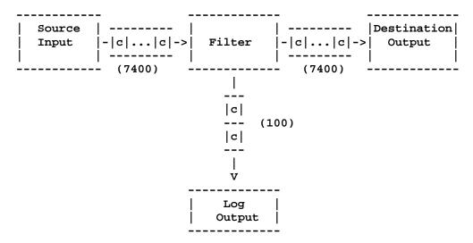
The numbers in parentheses are the maximum number of characters that can be in each buffer. With this structure, if most messages are passed to the destination, the rate at which messages flow through the MFM is determined by the processing rate of the slowest process. Thus, if the filtering process can keep up with the input and output processes, the message delivery rate is roughly the same for a modulated connection as for a direct connection.
