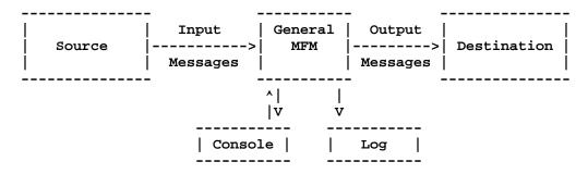
As in the OSIS modulator, the general modulator begins by applying a filter to a message. However, in the general modulator, if the message passes the filter, the message is transformed before it is passed to the destination.
