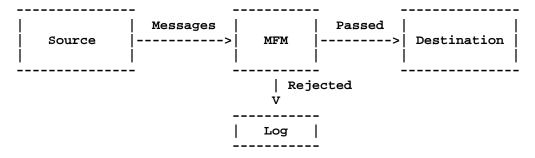
The modulator has been designed specifically to monitor the flow of security sensitive message traffic from the Ocean Surveillance Information System (OSIS) of the United States Naval Electronic Systems Command. The filter applies pre-defined security criteria to each message. Those messages that satisfy the security criteria are passed to the destination. All others are rejected and logged on an audit trail.
