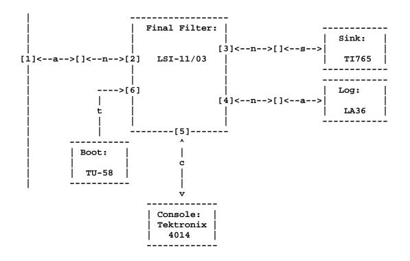
MESSAGE FLOW MODULATOR Cable Connections
