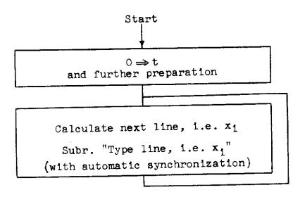
The test for the end of the table has been omitted in the above diagram. The results of the computation are stored per line at a number of addresses, reserved for the variables x; these addresses are to be regarded as working spaces for the computing main program and as "parameter addresses" for the subroutine "Type line", which is now given.
