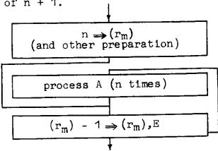
It often happens that a loop has to be passed through " $n-\frac{1}{2}$ " times, i.e. one part (process A) must be done n times, the other part (process B) only n-1 times. This is shown in the following flow diagram.
