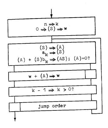
The scalar product is delivered in two words: the most significant half in the working space w, the least significant half in the S-register. The halves need not have the same sign!
