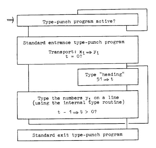
The test "t=0?" was introduced in order to type the very first line only once. The transport  $x_i \Rightarrow y_i$  is necessary because the one line still has to be typed while the main program is already engaged in the calculation of the new values  $x_i$  for the following line. The addresses for the numbers  $y_i$  are to be regarded as working space belonging to the type-program; it is strictly forbidden territory for the main program!
