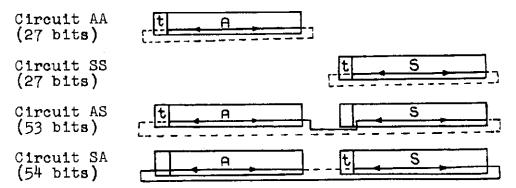
The sign digit of the first register named acts as "the sign digit of the circuit", in the diagrams it is indicated by t. We note that the sign digit of S is not included in the circuit AS.
