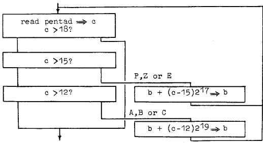
word the pair of bits describing A, B or C are to be stored on the immediate left of the pair of bits describing P, Z or E.
