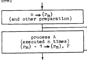
This diagram only applies to the case  $n \ge 1$ . Particularly in the case where the number n is a previously computed quantity, it often happens that the minimum value of n is = 0. Here we can use the last criterium E ("Extra Jump") for the counting jump and save a separate test for detection of n = 0 or the formation of n + 1.
