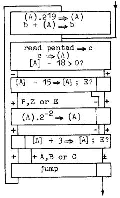
For the purposes of clarity we make use of a flow diagram to describe the procedure in the X1 program. Where relevant the content of the last sign register is shown by + or -. The question about equatity of signs is indicated by "E?". Conditional execution is explicitly shown by dividing the block in two by a vertical line.
