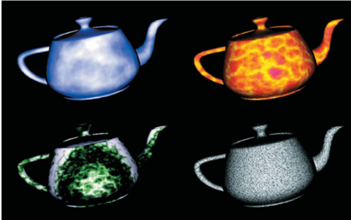
Figure 8.27 Teapots rendered with noise shaders (Clockwise from upper left: a cloud shader that sums four octaves of noise and uses a blue-to-white color gradient to code the result; a sun surface shader that uses the absolute value function to introduce discontinuities (turbulence); a granite shader that uses a single high-frequency noise value to modulate between white and black; a marble shader that uses noise to modulate a sine function to produce alternating “veins” of color. (3Dlabs, Inc.))
