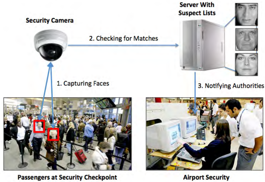
Figure 1.1: Data flow for an identification system; e.g. at an airport. Passenger faces are initially captured by a security camera as passengers pass through the security checkpoint. The security camera transmits each face to the server to be compared. If the server sees a match with any faces in its database, it notifies airport security.
