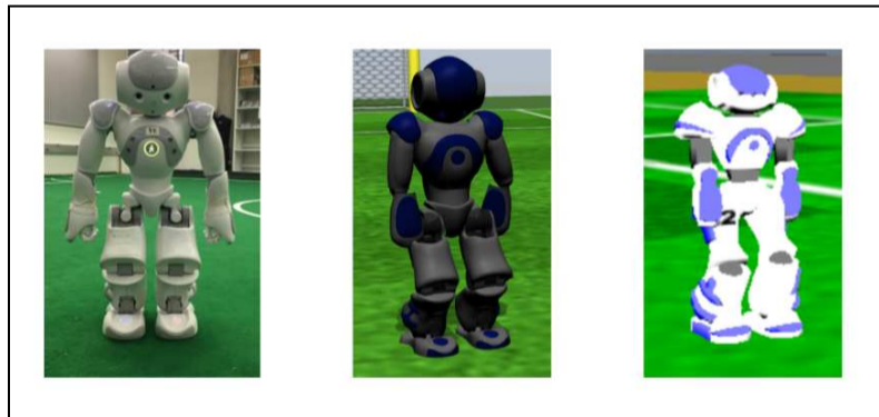
Figure 3: Walk policies learned within the Gazebo Simulator (center) and SimSpark Simulator (right) were successfully transferred to the SoftBank NAO robot (left). Walk policies learned within SimSpark were successfully transferred to the Gazebo simulator.
