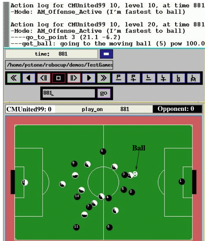
Fig. 6: The hierarchical extrospection tool. The terminal window at the top is displaying the high-level information for the agent with the ball (number 10 on the light-colored team) at the instant shown in the graphical display of the game. At level 10, only the agent’s active mode (“offense active”) is shown. At level 20, information about its high-level actions are also included. In this case, the agent is trying to intercept the moving ball at a specific point. Details about how this point was arrived at, as well as the resulting low-level action, the agent’s most recent sensory perceptions, and the agent’s current world state can be displayed by moving to a lower hierarchical behavior layer. On the control bar in the middle, the buttons labeled with a “P” are used to control which agent is being examined. The buttons labeled “L” are used to control at what layer it is being examined (“L/0” and “L/M” are shortcuts for the lowest and highest layers respectively).
