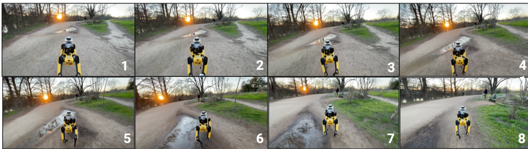
Figure 17: STERLING navigating around an unfamiliar terrain, specifically a “water puddle”, during the qualitative 3-mile off-road deployment.
