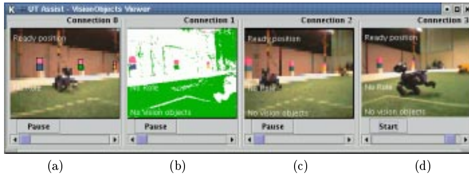
Figure 15: Several examples of visual data displayed in UT Assist. Part (a) contains a low-resolution image with vision objects overlaid on top. Part (b) shows a color segmented image. Part (c) contains a low-resolution image, and (d) contains a high-resolution image.
