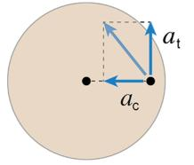
The centripetal acceleration is perpendicular to the tangential acceleration, so we apply the Pythagorean theorem, as follows, to find the magnitude of the total acceleration:
