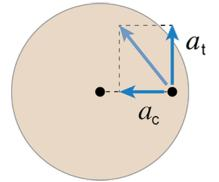
The centripetal acceleration is perpendicular to the tangential acceleration, so we apply the Pythagorean theorem, as follows, to find the magnitude of the total acceleration:
