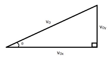
Recall that the sine function of an angle in a right triangle gives the opposite side divided by the hypotenuse. We can use this to write an equation to relate the angle, initial velocity, and the initial vertical velocity.
