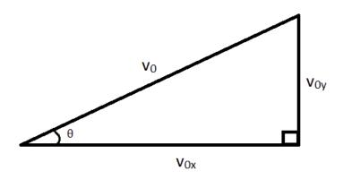
Recall that the cosine function of an angle in a right triangle gives the adjacent side divided by the hypotenuse. We can use this to write an equation to relate the angle, initial velocity, and the initial horizontal velocity.
