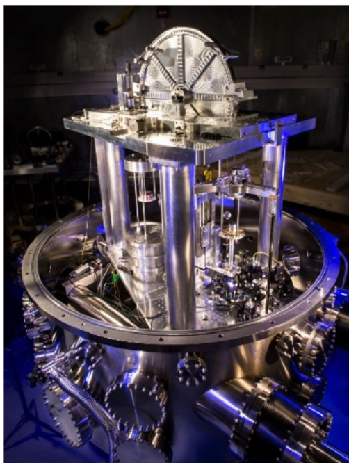
Figure 1.10 Redefining the SI unit of mass. The U.S. National Institute of Standards and Technology's Kibble balance is a machine that balances the weight of a test mass with the resulting electrical current needed for a force to balance it.
