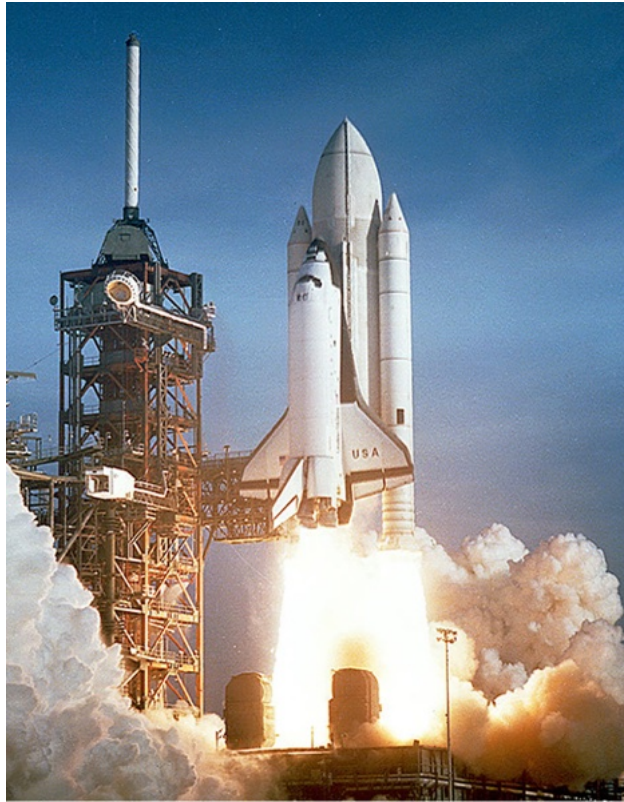
Figure 9.32 The space shuttle had a number of reusable parts. Solid fuel boosters on either side were recovered and refueled after each flight, and the entire orbiter returned to Earth for use in subsequent flights. The large liquid fuel tank was expended. The space shuttle was a complex assemblage of technologies, employing both solid and liquid fuel, and pioneering ceramic tiles as reentry heat shields. As a result, it permitted multiple launches as opposed to single-use rockets. (credit: modification of work by NASA)
