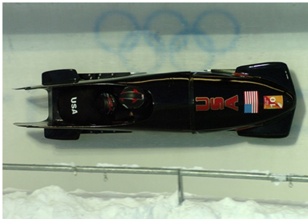
Figure 6.29 From racing cars to bobsled racers, aerodynamic shaping is crucial to achieving top speeds. Bobsleds are designed for speed and are shaped like a bullet with tapered fins. (credit: "U.S. Army"/Wikimedia Commons)
