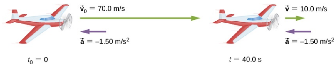
Figure 3.19 The airplane lands with an initial velocity of 70.0 m/s and slows to a final velocity of 10.0 m/s before heading for the terminal. Note the acceleration is negative because its direction is opposite to its velocity, which is positive.
