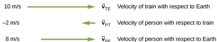
Figure 4.25 Velocity vectors of the train with respect to Earth, person with respect to the train, and person with respect to Earth.
