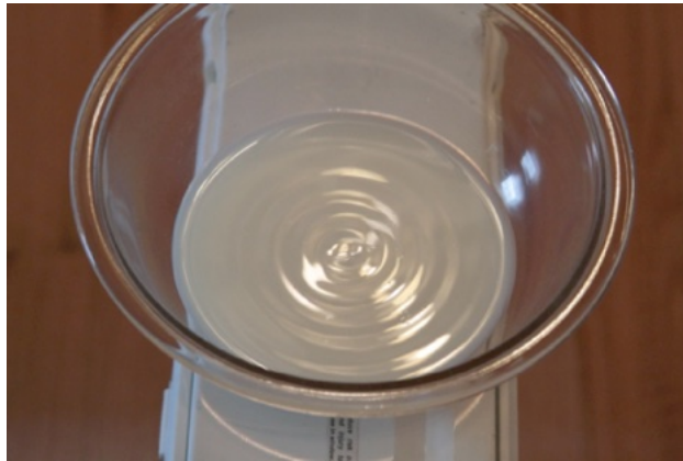
Figure 16.25 Standing waves are formed on the surface of a bowl of milk sitting on a box fan. The vibrations from the fan causes the surface of the milk to oscillate. The waves are visible due to the reflection of light from a lamp. (credit: David Chelton)
