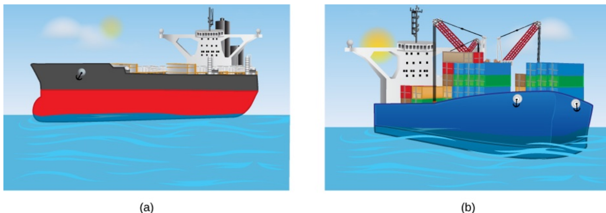
Figure 14.22 An unloaded ship (a) floats higher in the water than a loaded ship (b).
