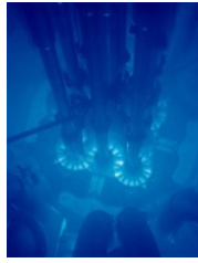
Figure 17.39 The blue glow in this research reactor pool is Cerenkov radiation caused by subatomic particles traveling faster than the speed of light in water. (credit: Idaho National Laboratory)
