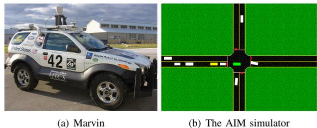
Fig. 3. The full sized autonomous vehicle and the AIM simulator in our mixed reality platform. The green rectangle in the middle of the intersection is a *proxy vehicle* representing the real world location of the autonomous vehicle. The white rectangles are virtual vehicles with reservations, while the yellow rectangles are virtual vehicles without reservations.
