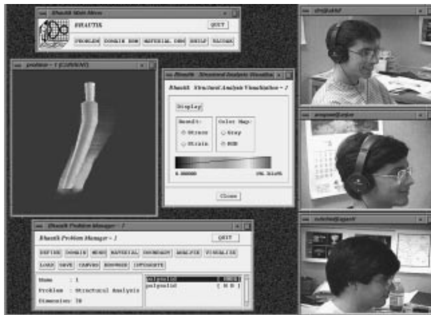
Figure 7: Stress Analysis Visualization – A designer uses Bhautik to analyse stress under loading patterns to optimize custom implant shape for an artificial implant for a human femur (top-left). The designers use video-conferencing for communication.
