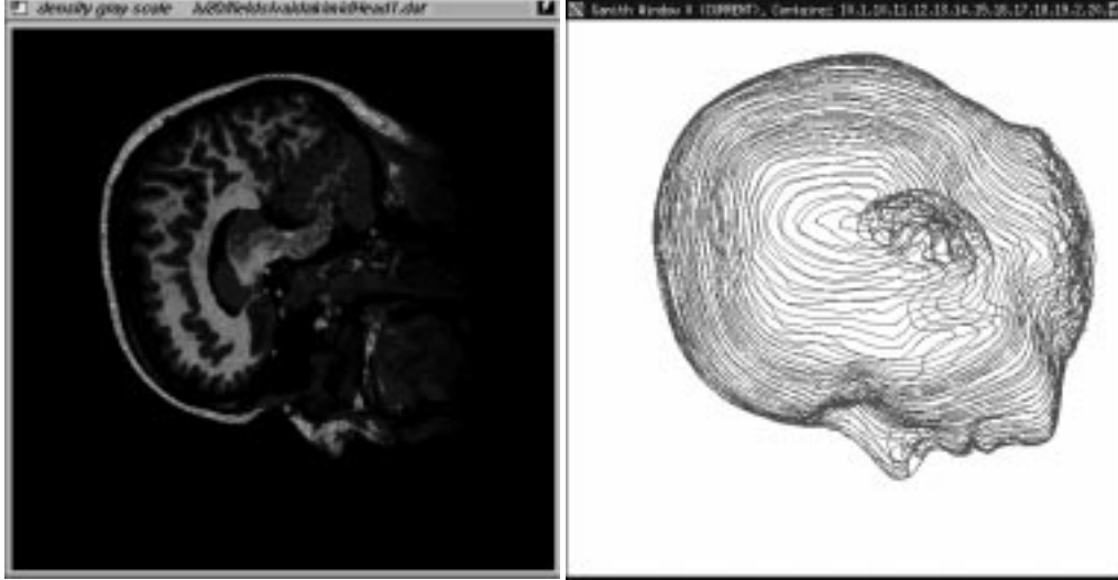
Figure 1: A Stack of C^1 Smooth Cubic Spline Contours which are Iso-Curves from a Stack of MRI Data Slices
