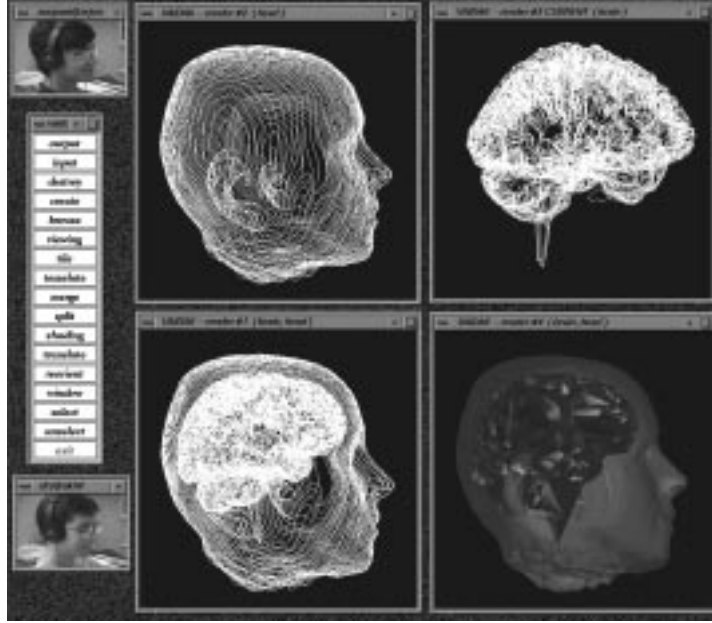
Figure 2: A Shared Visualization in SHASTRA of the Models of the Head and the Brain which are Iso-Surfaces from the Volume Cuberille MRI Data
