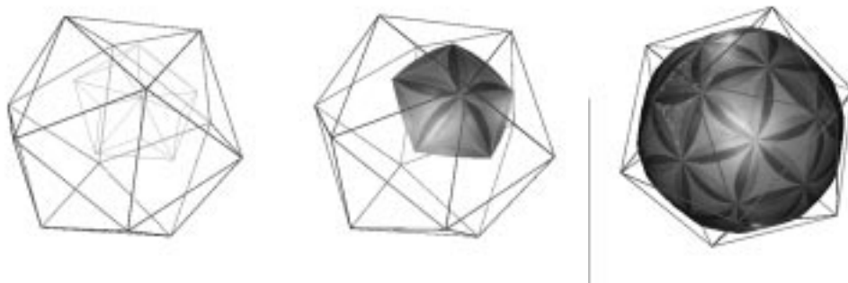
Figure 4.10: Corner Cuts, Inner Simplicial Hull and C^1 smooth A-patches
