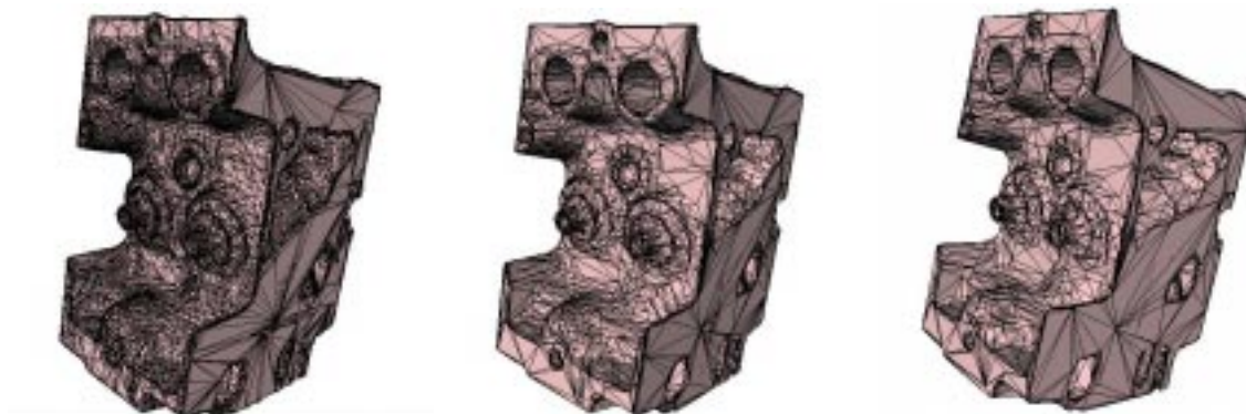
Figure 1.9 Three snapshots of geometric mesh simplification of an engine block
