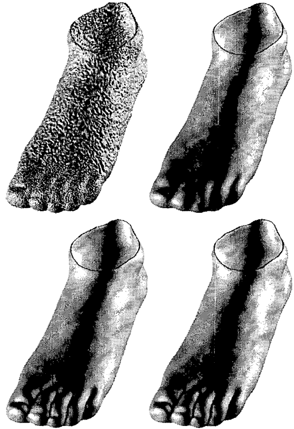
Fig 4.1: The left top figure is the initial geometry mesh. The right top figure is the faired mesh after 3 fairing iterations with uniform timestep t = 0.0011 . The left and right figures in the bottom row are the faired meshes after 3 fairing iterations with adaptive timestep and alternatively adaptive diffusion tensor with uniform timestep \tau_i = 0.025 , respectively.
