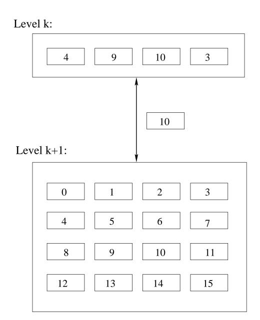
Smaller, faster, more expensive device at level k caches a subset of the blocks from level k+1.
