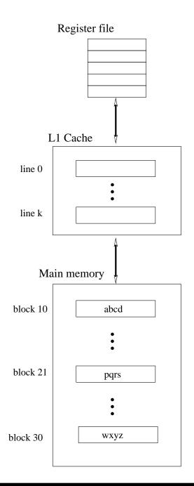
The tiny, very fast CPU register file has room for a small number of 8-byte words.
