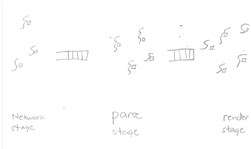
Figure 5.1: A multi-stage server based on the ownership pattern. In the first stage, one thread exclusively owns each network connection. In later stages, one thread is processing a given object at a time.
