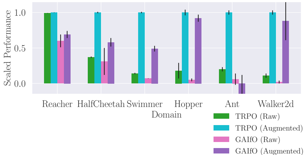
Figure 7.2: Quantitative exhibition of the importance of an augmented state space for high performance on six MuJoCo domains for GAIfo and TRPO . Mean and standard deviations are over 100 policy runs. The results are brought here as we seek the RIDM to operate over raw state space and to show how challenging it is to learn when raw state space is considered compared to augmented space. Both methods use a neural network parameterized policy.
