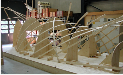
Figure 3: Assembling screw-laminated beams for a timber rib shell prototype based on a 2-pattern of geodesics. Image courtesy IBOIS, the timber construction lab at EPF Lausanne.
