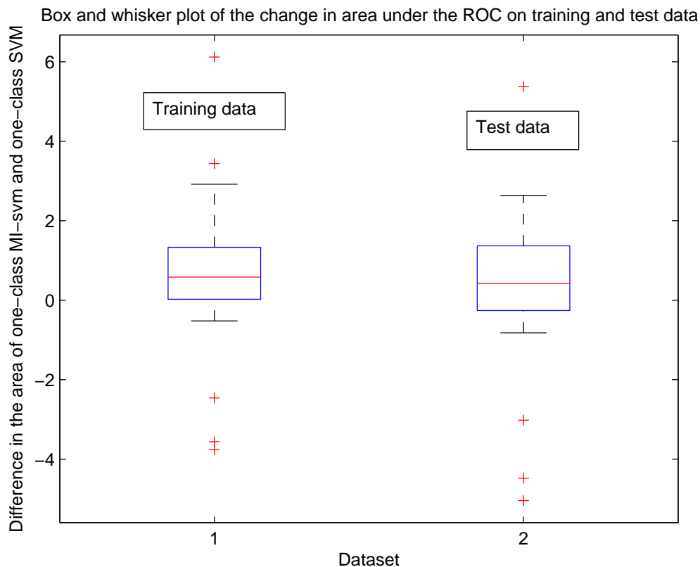
Figure 3: A box and whisker plot of the difference in the area under ROC for the two methods. The mean and lower quartile are above zero for both test and training data implying that the MI constraint does improve the area under the ROC for most categories
