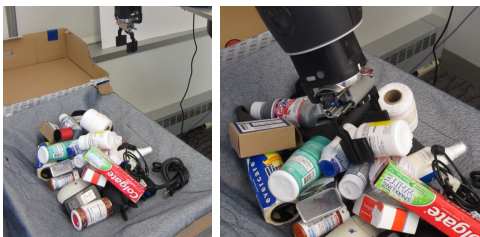
Fig. 1. Our algorithm is able to localize and grasp novel objects in dense clutter.
