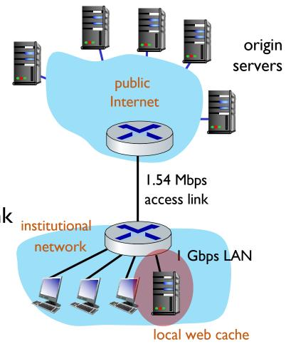
lower average end-end delay than with 154 Mbps link (and cheaper too!)
