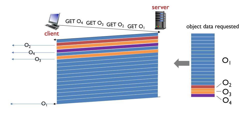
O<sub>2</sub>, O<sub>3</sub>, O<sub>4</sub> delivered quickly, O<sub>1</sub> slightly delayed
