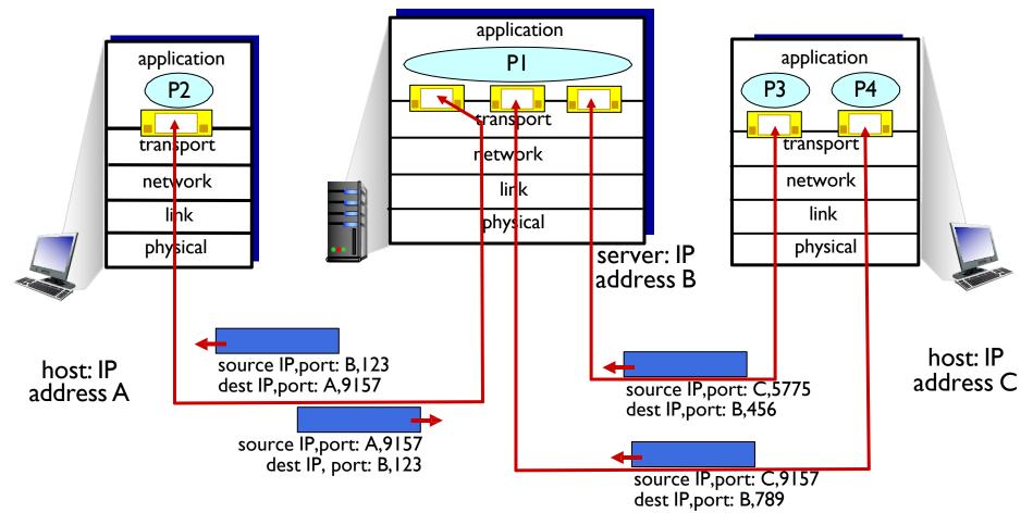
Three segments, all destined to IP address: B are demultiplexed to different sockets
