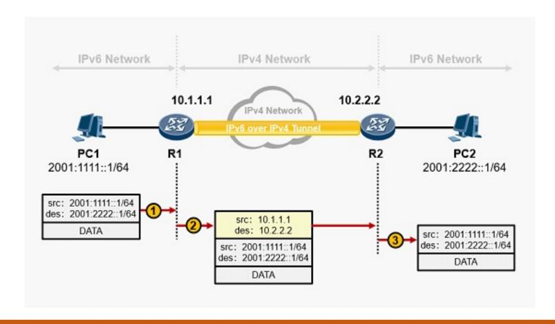
Tunnel is implemented by encapsulating IPv6 datagram with IPv4
