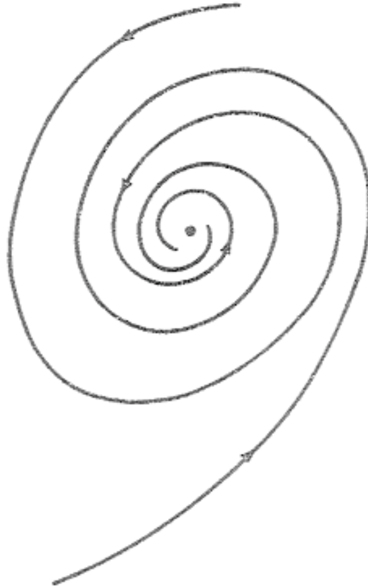
FIG. E. Spiral sink: B = \begin{bmatrix} a & -b \\ b & a \end{bmatrix} , b > 0 > a .
