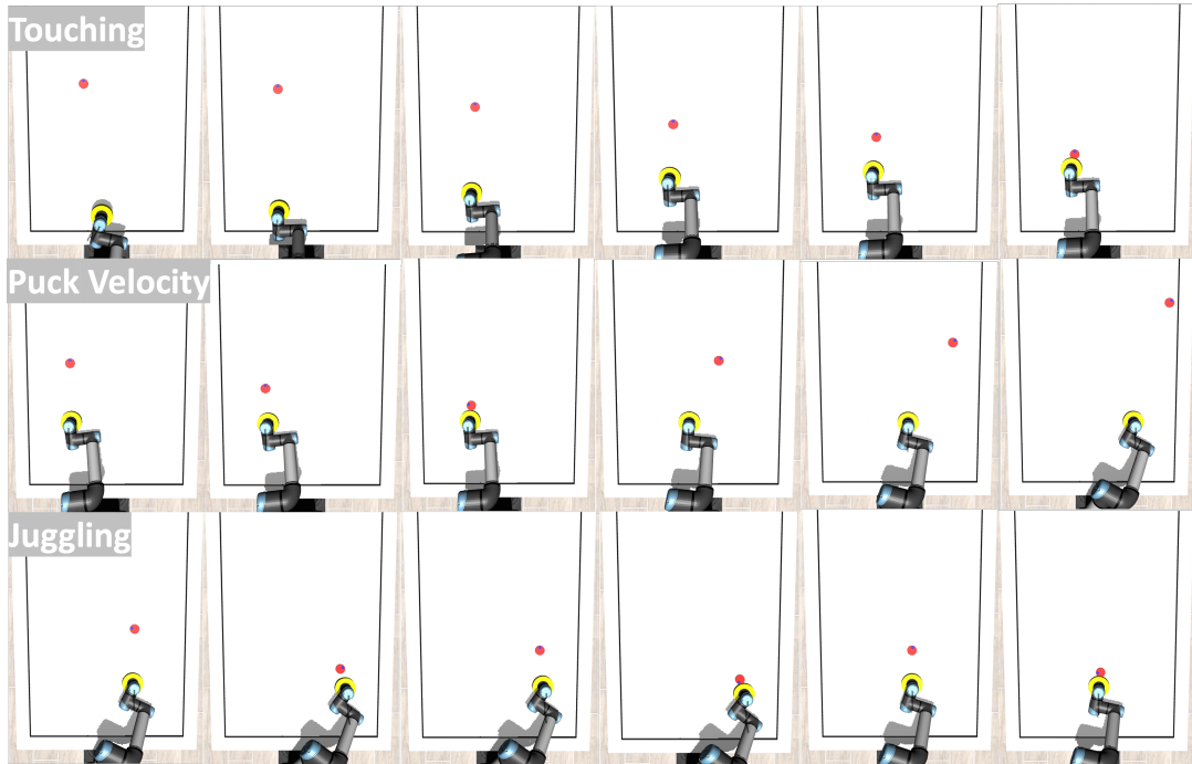
Fig. 6: Execution rollouts in Robosuite simulator. The puck is circled in red for emphasis. Policies are trying to touch the puck, hit the puck with a minimum upward velocity, and juggle the puck.
