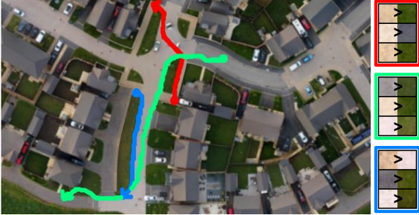
Fig. 5: Examples of several paths planned using our method in an urban unseen environment and their corresponding preference contexts. Here, we visualize the large scale of these simulated deployments, and the diversity of visual terrain appearances.
