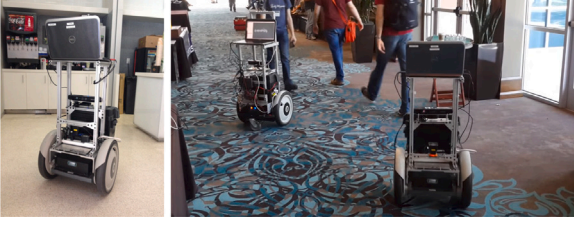
Fig. 4. The robot platform used in experiments, called BWIBot [5]. The platform is based on a Segway RMP, and is equipped with sensing capabilities, including laser-based range finding for localization, voice recognition for human-robot dialog, and RGB-depth sensors for human detection and obstacle avoidance. The right is a picture of two BWIBots running at the venue of the Twenty-Ninth AAAI Conference on Artificial Intelligence in Austin, TX.
