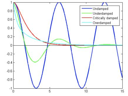
• Underdamped (D<0,  $\zeta$ <1)  $x(t) = e^{-\zeta \omega_0 t} (A \cos(\omega_d t) + B \sin(\omega_d t))$  $\omega_d = \omega_0 \sqrt{1 - \zeta^2}$
