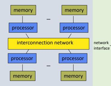
Massively Parallel Processor (MPP) Many, many processors
