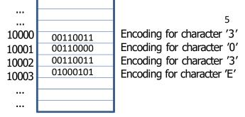
A byte is the smallest unit of storage a programmer can address. We say that the memory is *byte-addressable*.
