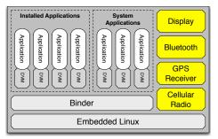
Figure 1: The Android system architecture
