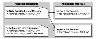
Figure 5: Eavesdropping on unprotected intents
