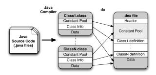
Figure 2: Compilation process for DVM applications
