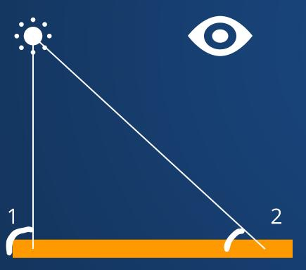
Is based on the cosine of angle between the light and the surface.
