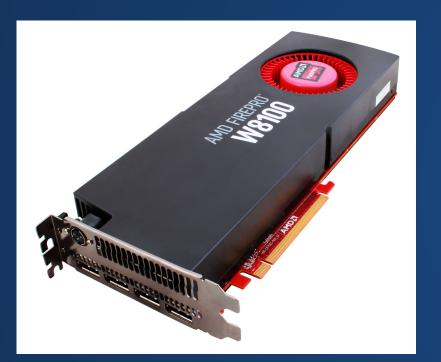
GPUs are processing units which specialize in the types of computations needed for graphics.
