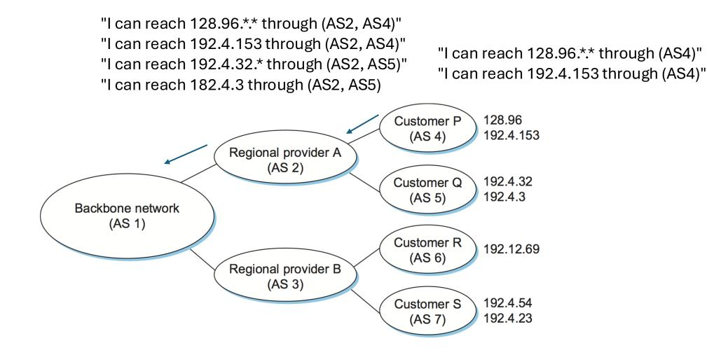
"I can reach 128.96.\*.\* through (AS1, AS2, AS4)" "I can reach 192.4.153 through (AS1, AS2, AS4)" "I can reach 192.4.32.\* through (AS1, AS2, AS5)" "I can reach 182.4.3 through (AS1, AS2, AS5)
