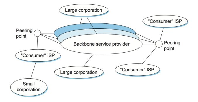
Each "Autonomous System (AS)", represented by ellipses here, can do whatever they want internally. They can be connected in complex topologies\*. As long as they all speak BGP, the internet works\*
