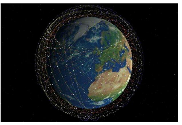
Covers the entire planet with a low latency network that is also lower capacity compared to fiber network, primarily because of earth-to-space communication bottleneck
