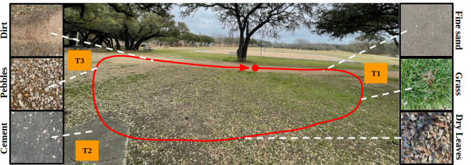
Fig. 7: Outdoor Evaluation Environment. Various traversed terrain types are highlighted, and the evaluation trajectory is illustrated in red. T1, T2, and T3 indicate the distinct turns in the trajectory.
