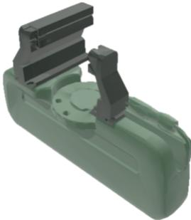
Fig. 4. BioGIGA gripper design. For a precision grip the thumb gripper finger moves to the inside of the front of the palm and aligns in between the index and middle finger. For a power grasp configuration the thumb is aligned with the index finger but has a small time delay of 0.1-0.3 s and an increase in the gripper force that is introduced by modifying the velocity and stiffness of the thumb gripper.
