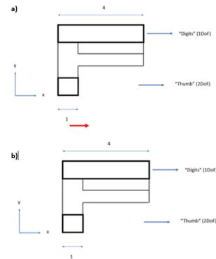
Fig. 2. Our approach using the BioGIGA gripper design based on human physiological behavior. a) Shows the precision grasp pattern in which there is an horizontal translation of the thumb gripper finger. b) Power grasp configuration in which the thumb is aligned with the index finger.
