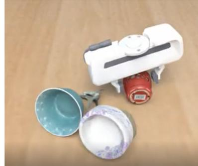
Fig. 6. BioGIGA new gripper configuration for a grasping task using a power pattern in the simulation environment
